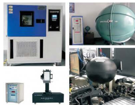
检测设备 Inspection Equipment (Humid/Temp Test, distribution photometer, Sphere,)
